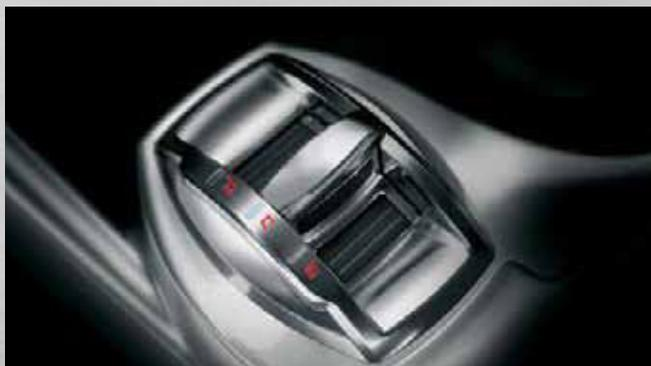
Fahrdynamikregelung Alfa Romeo D.N.A., 3-stufig einstellbar (Dynamic / Natural / All Weather)<sup>1</sup>
