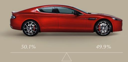
By tucking the 6.0-litre V12 engine behind the centreline of the front wheels and mounting the six-speed Touchtronic 2 transaxle at the rear, not only are the Rapide S major masses concentrated within the
