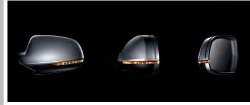
Electrically adjustable door mirrors with integrated indicators
