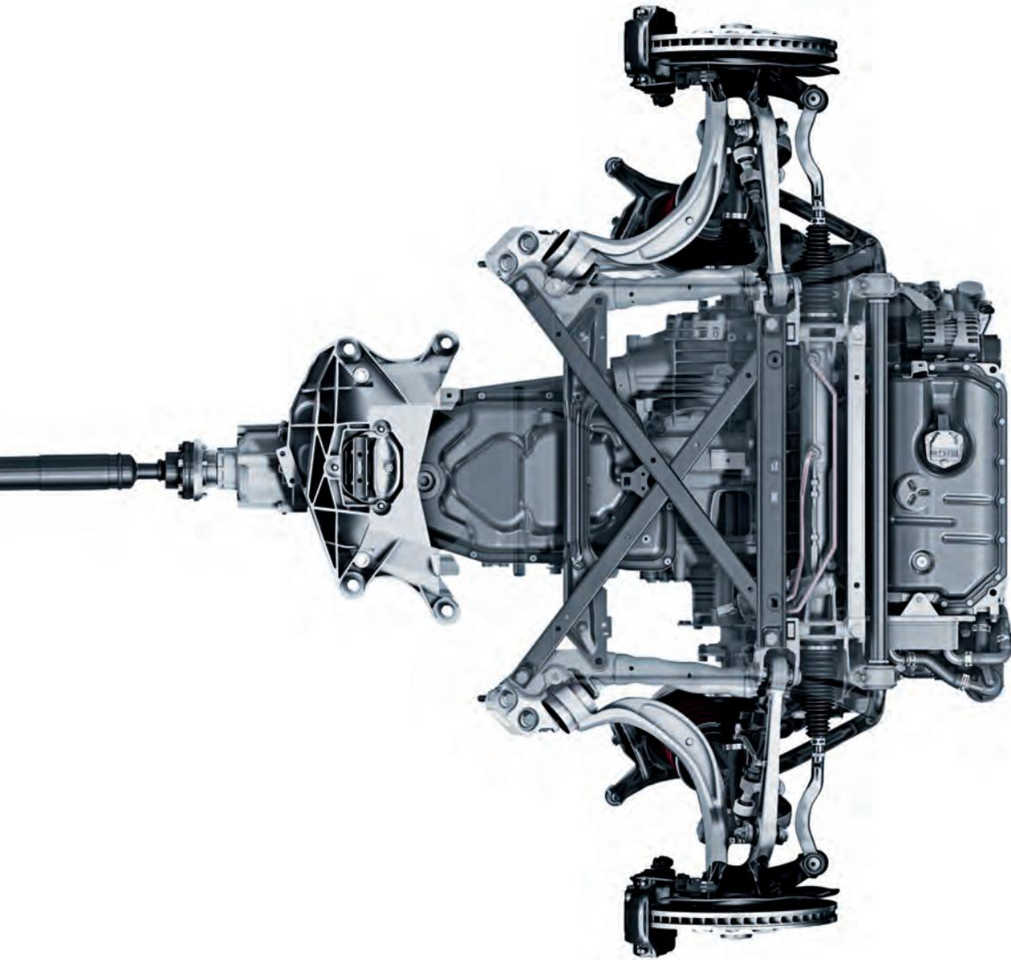
In the Audi A5 Cabriolet, asymmetric dynamic torque distribution continuously distributes drive power between the front and rear axles, depending on weather conditions, road surface and gradient. This leads to greater flexibility and an enhanced, sportier drive.
