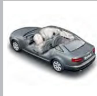
Driver/front passenger two-stage airbags with front passenger airbag deactivation
