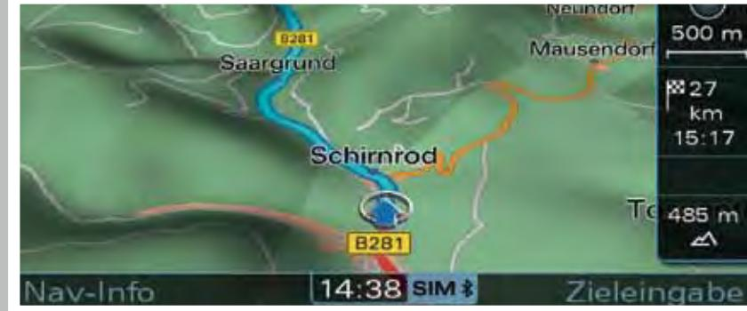
3D topographical mapping display (part of HDD Navigation)
