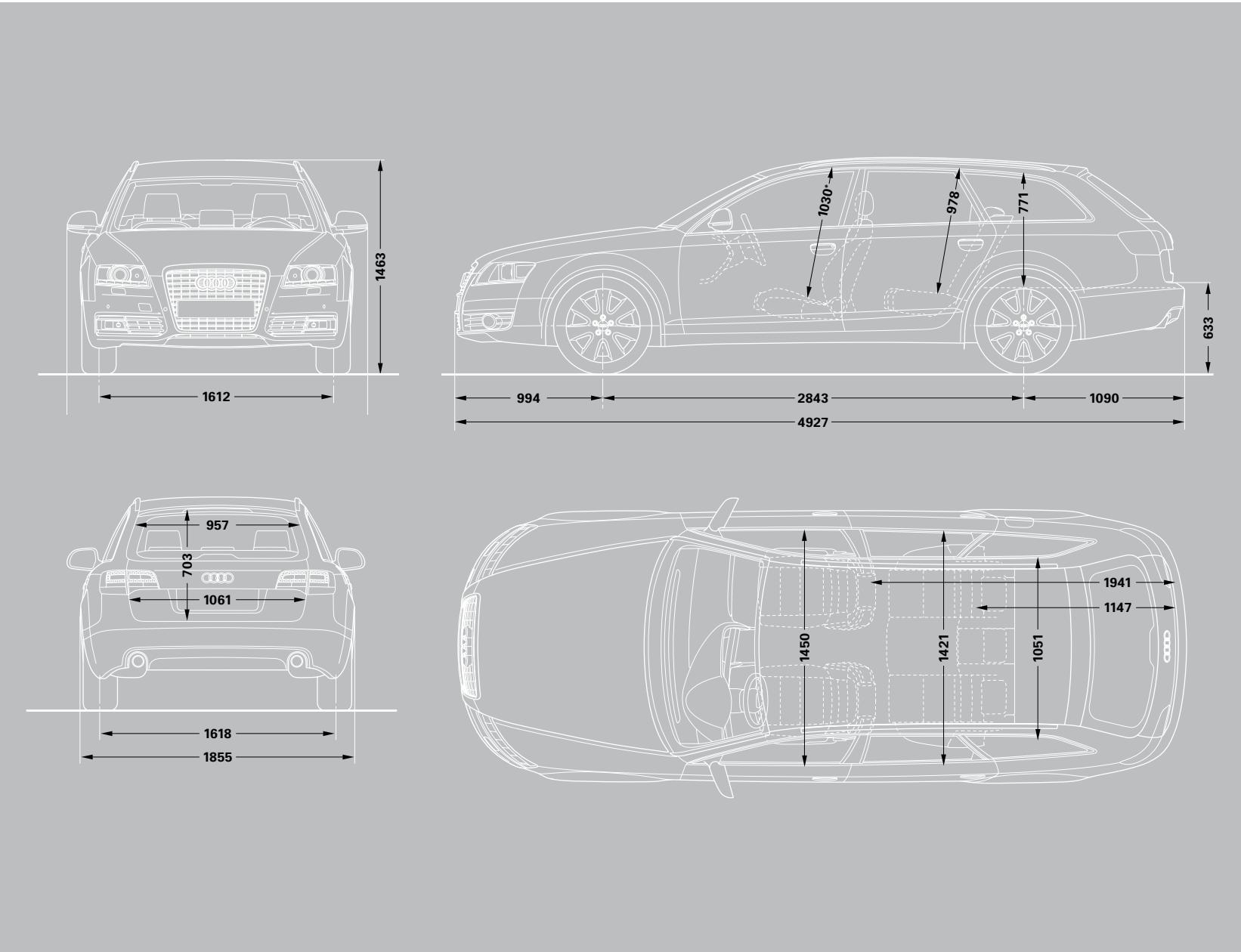
Dimensions were measured with vehicle at unladen weight.
