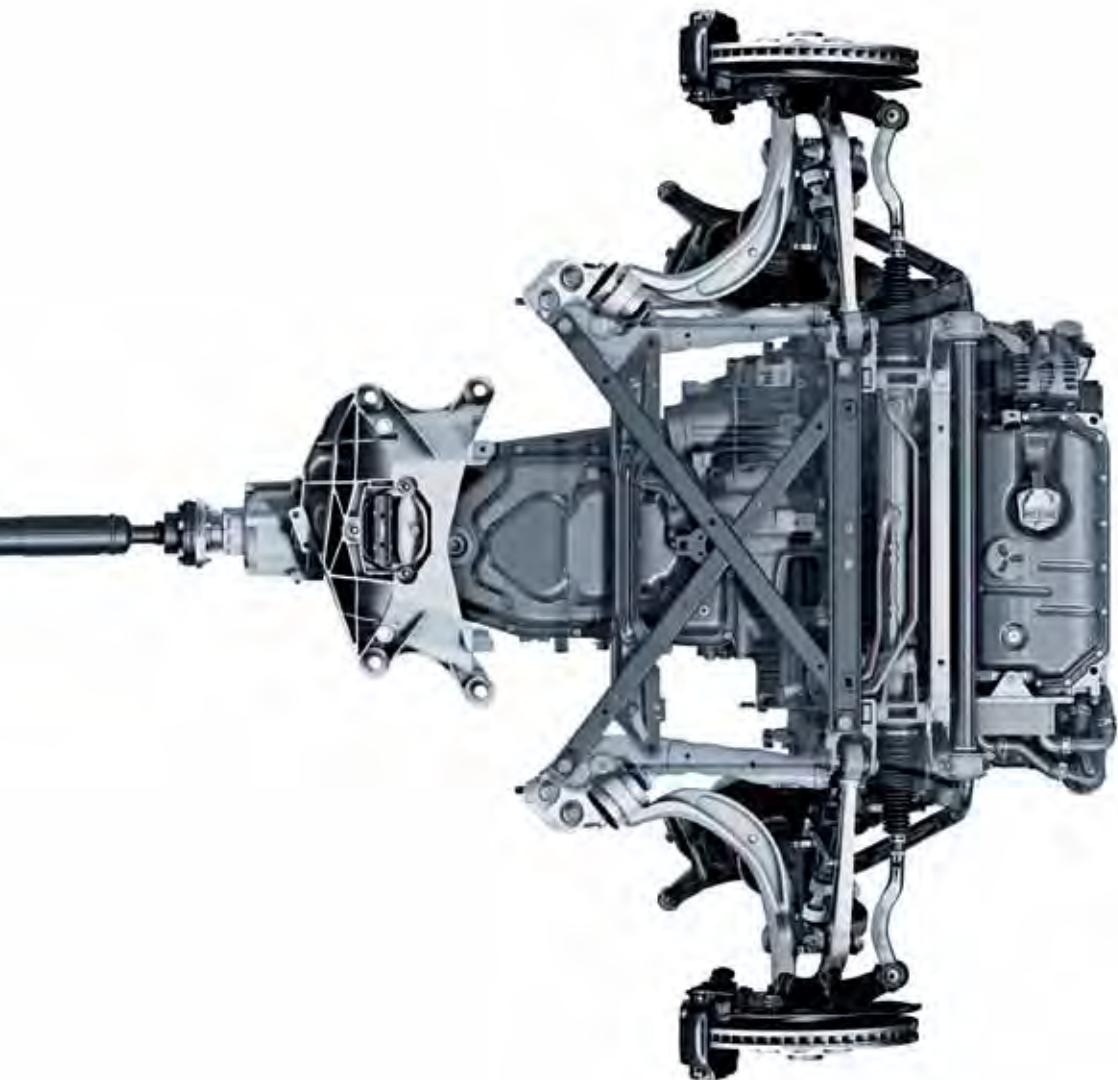
In the Audi A6, asymmetric dynamic torque distribution continuously distributes drive power between the front and rear axles, depending on weather conditions, road surface and gradient. This leads to greater flexibility and an enhanced, sportier drive.
