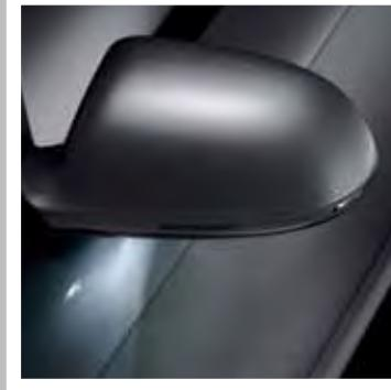
Exterior lighting integrated into door mirrors
