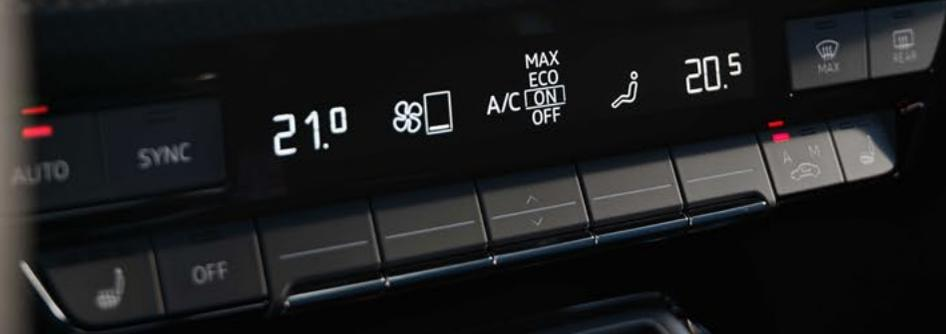
The climate control panel features a digital display showing '21.0' on the left and '20.5' on the right. Between the numbers are icons for fan speed, air recirculation, and a person icon. The text 'MAX ECO' is positioned above 'A/C', which is above 'ON' and 'OFF'. To the right of the display are two buttons labeled 'MAX' and 'REAR'. Below the display is a row of physical buttons, including 'OFF', 'AUTO', and 'SYNC'.
