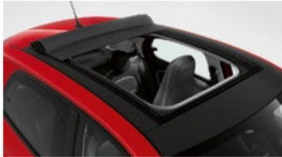
Faltdach in Stoff elektrisch (forfour) [E55]
