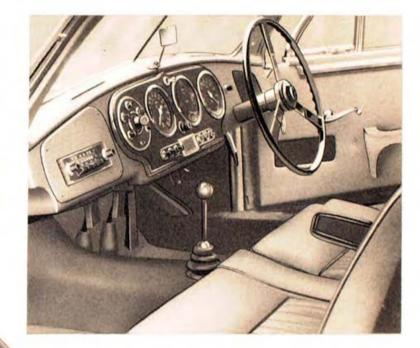
THE ATTRACTIVE INTERIOR OF THE DB2. The loxurious front seats give full three-seater accommodation, and have folding centre arm-rest. Excellent huggage accommodation is provided behind the seats. Full range of instruments includes speedometer, mileage and trip recorders, rev. counter, clock, petrol and oil capacity gauges, oil pressure gauge, coolant thermometer and ammeter. Air conditioning and demisting equipment and windscreen washers are standard. (Radio extra.)
